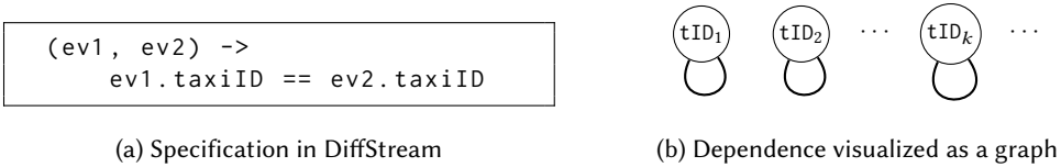
Fig. 4. Example specification in DiffStream for the taxi example. Taxi events with the same taxiID are dependent.
